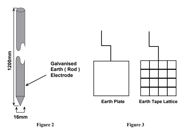
The galvanised earth electrode above is generally sufficient for a domestic installation. The ETCI Rules cover more specific requirements for types of earth electrode.
