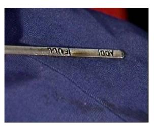
This can be caused by worn piston rings which let oil into the combustion chamber.
