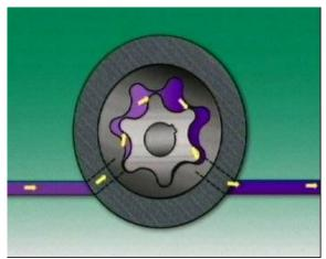
forces oil into the pump, and it fills the spaces between the rotor lobes.
