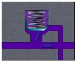
An oil pressure relief valve stops excess pressure developing. It's like a controlled leak, releasing just enough oil back to the sump to regulate the pressure of the whole system.
