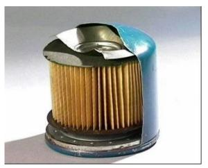
Normally all oil goes through the filter before it gets to the engine, but if the filter clogs up, it can starve an engine of oil.
