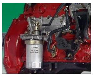
circulates through tubes in the cooler, and oil fed from the lubrication system surrounds the tubes. As the coolant circulates, heat is removed from the oil.
