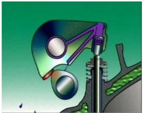
between moving parts, but not so thin that it will be forced out from between them. If it is forced out, parts will be left in direct contact and they'll be damaged.
