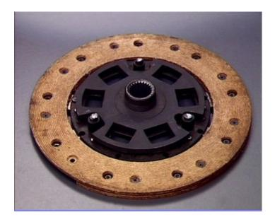
The driven plate has a pair of friction facings, of wire-reinforced asbestos-free composition, carried on waved spring steel segments, which are riveted to a steel disc.
