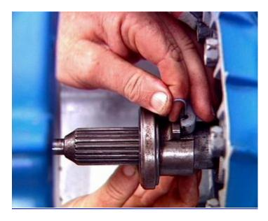
The bearing carrier locates on the clutch release fork. Moving the fork brings the bearing thrust face into contact with the pressure plate fingers. This causes the bearing to rotate, and absorb the rotary motion of the fingers, against the linear motion of the fork. The bearing is packed with lubricant during manufacture and requires no periodic maintenance during its service life.
