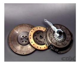
The clamping force on the friction facings is provided by the diaphragm spring. Unloaded, it is a dished shape. As the pressure plate cover tightens, it pivots on its fulcrum rings, and flattens out to exert a force on the pressure plate, and the facings.
