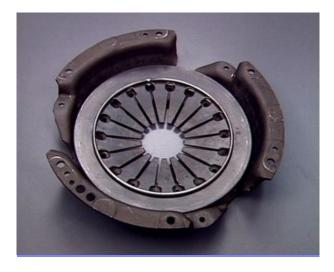
It consists of a pressed steel cover, a pressure plate with a machined flat surface, a number of spring steel drive straps, and the diaphragm spring.
