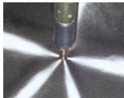
Uniform spray pattern with clean injector.
