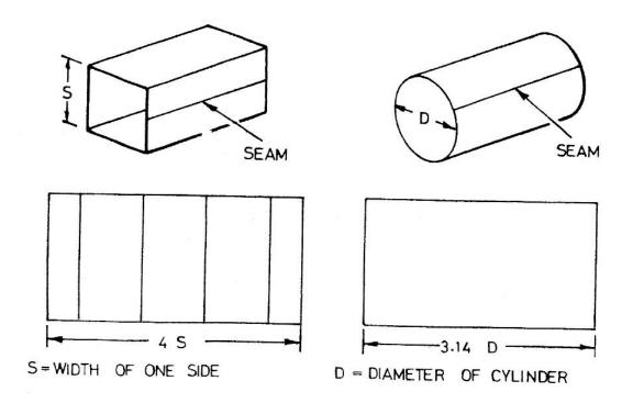
Layout or development generally refers to the method of developing the lines which form the pattern. The common methods of layout or development are:
