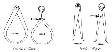
A calliper is usually used in one of two ways. Firstly, take the dimension of the component using an inside or outside callipers, and measure the distance between the calliper legs using a steel rule.
