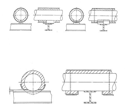
*Note:* Where cladding has to be cut away it shall fit closely to the pipe and be completely waterproof.
