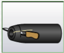
Cut reducer to size - allow compression of 5mm at each end. Slit fitting on the flat side
