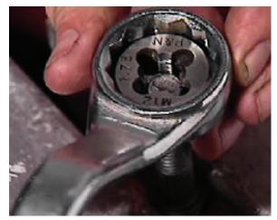
The die nut is more common in the workshop. It's hexagonal to fit a spanner and it's mostly used to clean up threads that have been damaged.
