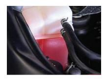
• For each 10 kPa increase in the radiator cap operating pressure, it will increase the boiling point of the coolant by 2°C (1 PSI for each 3°F).
