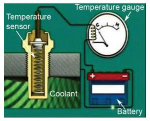
Indicators that measure coolant levels can give warning if the level falls too low.
