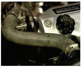
All hoses are subject to hot coolant and high under-bonnet temperatures and they can deteriorate and fail.
