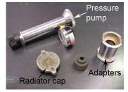
If you need to replace a pressure cap, use only a cap with the correct recommended pressure. If a cap with a lower pressure rating is fitted, it will lower the boiling point of the coolant. Alternatively, a higher rated cap will increase the boiling point.
