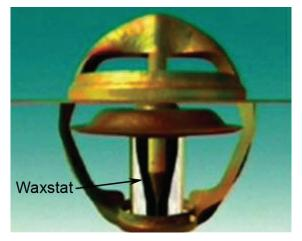
It is a valve that operates according to coolant temperature. When coolant is cold a spring holds the valve closed.
