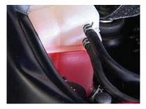
• For each 10 kPa increase in the radiator cap operating pressure, it will increase the boiling point of the coolant by 2°C.
