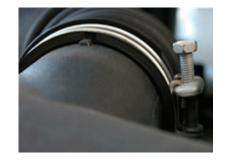
Banded or screw-type clamp. Also adjusted with a screwdriver.
