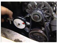
There are a number of different types of tension gauges. Follow the operating instructions on the tool. If you don't have a tension gauge, you can estimate the tension by pushing the belt inwards with your hand. If it's correctly tensioned, you should be able to deflect the belt about 1.25 centimetres for each 30cm of belt (half an inch for each foot).
