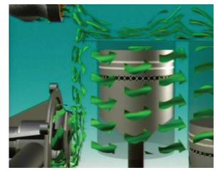
*Air cooling* is common on smaller internal combustion engines. Some engines use cooling fins. Their design makes the exposed surface area as large as possible which allows more heat energy to radiate away and be carried off in convection currents in the air. Some engines also use a fan to direct air over the fins.
