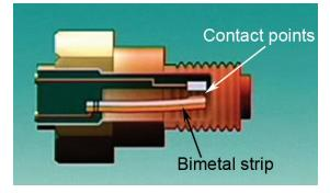
As the strip changes shape it can be designed to complete a circuit and a resulting electrical signal can then do a range of tasks or it might have a mechanical effect simply opening a passageway.
