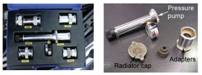
• If you need to replace a pressure cap, use only a cap with the correct recommended pressure. If a cap with a lower pressure rating is fitted, it will lower the boiling point of the coolant. Alternatively a higher rated cap will increase the boiling point.
