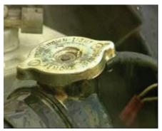
In a recovery system the hot coolant flows out into an overflow container. As the engine cools, coolant contracts and pressure in the radiator drops. Atmospheric pressure in the overflow container then opens a second valve, a vacuum vent valve and overflow coolant flows back into the radiator.
