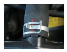
Wire clamp. This spring clamp is not adjustable and is fitted and removed with special hose clamp pliers, which have grooved jaws.
