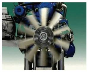
When an engine is mounted longitudinally, its fan is usually mounted on the water pump shaft. The drive belt then turns the water pump and fan. Some use a hydraulic link from the power steering system. Fan blades can be rigid or flexible. Rigid blades tend to be noisy and use more energy. This noise can be reduced by using irregular spacing of the fan blades. Some vehicles use a shroud to direct all of the air that the fan moves through the radiator core.
