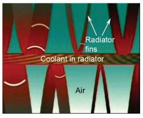
It can be made of sheet metal or hardened plastic. The radiator has 2 tanks and a core. The materials used in the radiator must be good heat conductors like brass or copper. Brass and copper are often used for tanks combined with a copper core.
