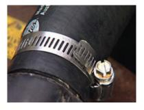
Gear or worm-type clamp. Adjust with a screwdriver.
