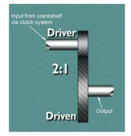
A manual transmission allows the driver to directly vary the gear ratio between the engine and the driving road wheels. This allows engine torque to be varied to suit load and speed requirements.
