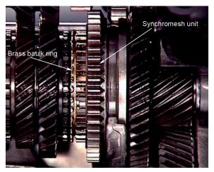
When first gear is selected, the engagement sleeve locks the first gear to the secondary shaft. When the clutch is released, the drive is transferred through the fixed first gear on the primary shaft, to the locked gear on the secondary shaft. The secondary shaft rotation transfers the drive through the main drive pinion to the final drive ring gear and the differential case.
