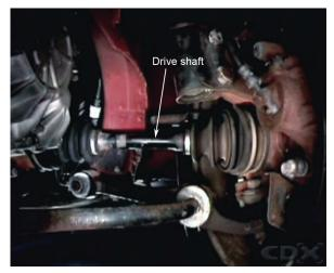
A short inner stub shaft is splined to the differential side gear and an outer stub shaft is splined to the front wheel hub. Each stub shaft has a yoke, or housing, to accommodate a universal joint, at each end of a connecting intermediate shaft.
