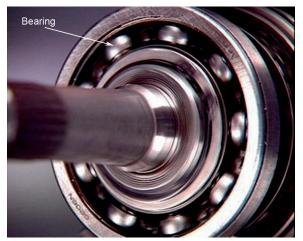
Thrust loads are applied along the length of the components, so the bearing must cater for side thrusts. In many cases these loads are combined and some bearings designed for radial loads will also accept light thrust loads. This applies to most ball bearings.
