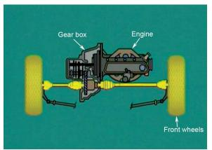
In this case the engine crankshaft transaxle shafts and drive shafts all rotate in-line which simplifies the final drive arrangement. Mounting the engine longitudinally means the drive must be turned through ninety degrees. A crown wheel and pinion is commonly used for this purpose.
