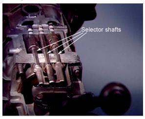
A short lever on the other end of the shaft is located in a selector gate, formed by slots in the three selector shift rails. They are supported in the casing and are moved backwards or forwards by the lever. One rail moves to engage first or second gear, another serves to engage third or fourth and the other operates fifth or reverse.
