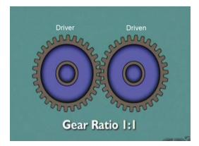
The transmission also provides a means of reversing the vehicle. And it has a neutral position, which disconnects the engine from the driving wheels. When two gears are in mesh, one is a driven or "output" gear. The other, providing the turning action, is the driver or "input gear". Gear ratio calculation formula: Driven Driver
