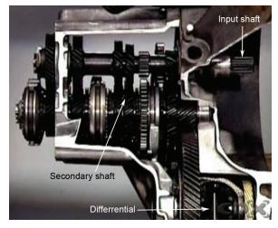
Each pair has one gear fixed to the primary shaft and one free to rotate on bearings on the secondary shaft. An engagement sleeve and hub, with a synchromesh unit facing each gear, is on the secondary shaft between first and second and similarly between third and fourth. The engagement sleeve moves to engage the dog teeth of the relevant gear when a gear is selected. This locks the gear to the shaft, so drive can be transmitted.
