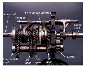
These gears mesh with mating gears on the main shaft, or output. These main shaft gears are supported on bearings on the shaft. They can rotate without turning the output. Each main shaft gear has an external toothed section on one side. The teeth face an internallytoothed engagement sleeve located on a central hub, which is itself splined to the main shaft.
