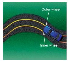
Note: Inner wheel has smaller angle than the outer wheel.
