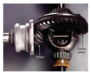
The ring gear is bolted to the case, so when it rotates, so does the case and the differential gears inside it. The two smaller bevel gears, or pinions, are mounted on a driving pin which passes through the case. Two side gears mesh with the pinions and are in recesses in the differential case. The drive shafts are splined to these side gears.
