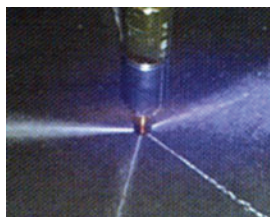
Poor spray pattern with clogged injector.
