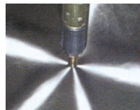
Uniform spray pattern with clean injector.
