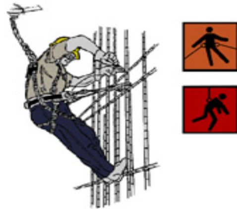
Fig 2 Harness attached to secure anchor point
